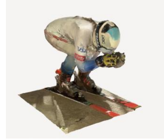
Figure 3. Raw 3D scan output of the tuck position captured using Polycam. This unprocessed mesh served as the starting point for model cleanup and aerodynamic simulation workflows.
